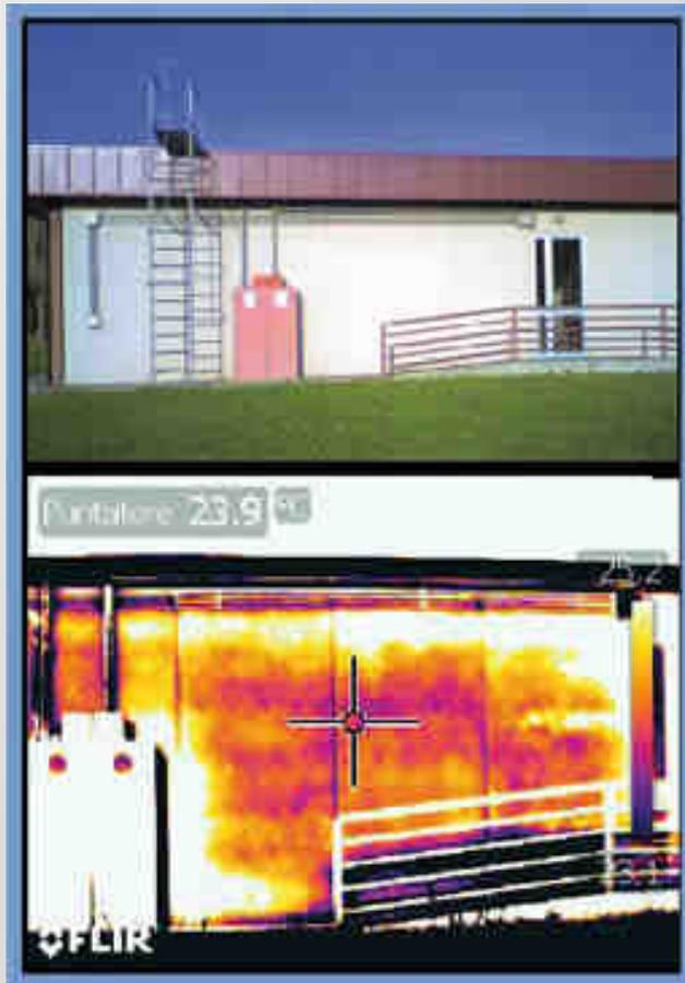
If we observe the images we see that there are high heat loss and this is an indicator that communicates the absence of insulation on the perimeter walls. It is needless remembering that to an increasing heat loss corresponds an increase of the fuel that we have to burn to maintain a good temperature inside and thus it increases the emissions into the atmosphere.
