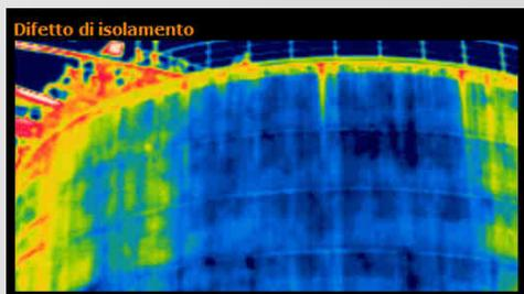
**TANK CONTAINING AMMONIA: INSULATION FAULT (2)**
